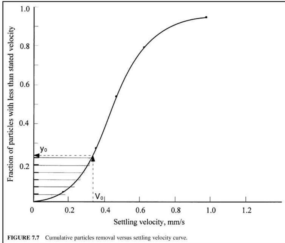
The settling velocity distribution for a suspension sample can be determined from a column settling test. The data obtained from the test can be used to construct a cumulative settling velocity frequency distribution curve, as shown in Fig. 7.7.
