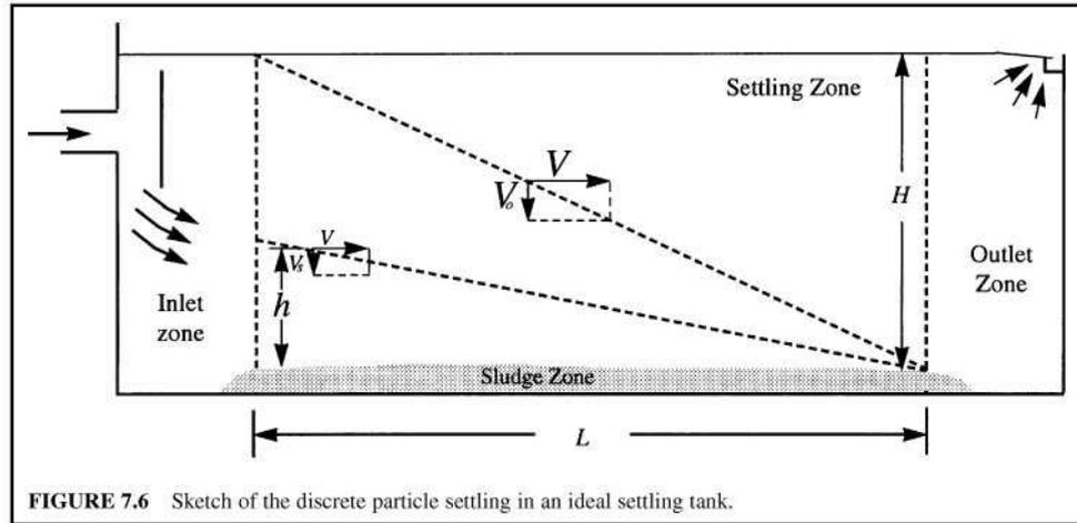
In the design of clarifiers, a particle terminal velocity  $V_0$  is used as a design overflow settling velocity, which is the settling velocity of the particle which will settle through the total effective depth  $H$  of the tank in the theoretical detention time. All particles that have a terminal velocity ( $V_s$ ) equal to or greater than  $V_0$  will be removed. The surface overflow rate of wastewater is (Stoke's law)
